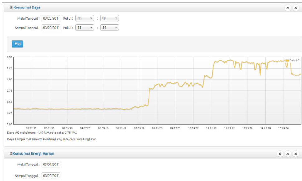
Figure 4. An example of energy consumption real-time monitoring at the Rectorate building 3 rd Fl. (Source: http://sinergi.ui.ac.id/new_rektorat/ )
