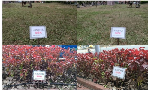
Figure 7. Soil improvement test of treated sludge (left: experimental test, right: control test)
