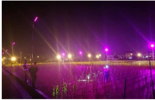
Figure 15. Luminance measurement in a simulated water bamboo field and an actual water bamboo field
