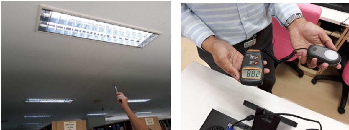
Figure 3. Field illuminance measurement
