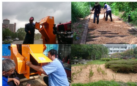
Figure 8. The crushing process and application of tree branches (left: crushing process, rihgt: paving and laying garden)
